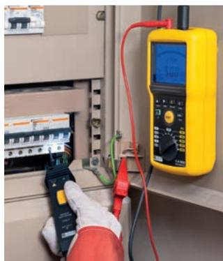
Insulation failure may lead to arcing between two points involving sparks which could set light to the materials around the point of failure.
