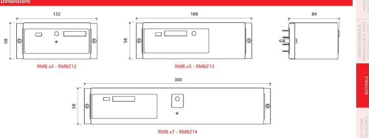
(\*) Models with manual operating lever (optional) are provided with a hole at the front giving access to the lever. The position of the data plate holder and the mechanical optical indicator can vary depending on the version.
