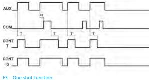
The control signal ("COM", 1B terminal) resets the time "t", on drop-out.
