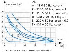
110 Vac - 5 A – Cos $\phi$  = 0.7: 5 x 10<sup>5</sup> operations 220 Vac - 3 A – Cos $\phi$  = 0.7: 5 x 10<sup>5</sup> operations 440 Vac - 0,2 A - Resistive: 5 x 10<sup>5</sup> operations
