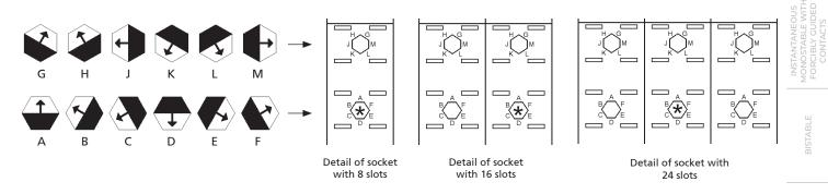
\*: receptacle to be left free in the event that the relay is fitted with an antirotation pin.
