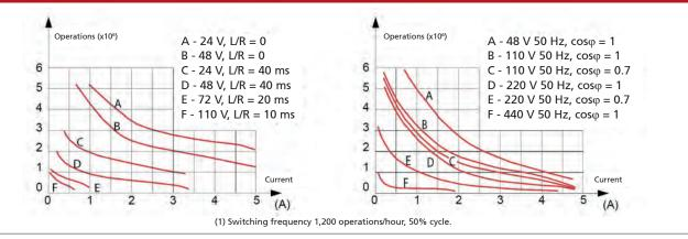
Examples of electrical life expectancy 48 Vdc - 5 A - L/R = 10 ms : 5 × 10<sup>5</sup> operations 80 Vdc - 5 A – Resistive : 5 × 10<sup>5</sup> operations 110 Vdc - 0,5 A - L/R = 10 ms : 5 × 10<sup>5</sup> operations
