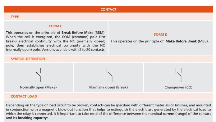
• NOMINAL CURRENT: The current that can flow through a contact for an indefinite period of time without the contact suffering damage.
