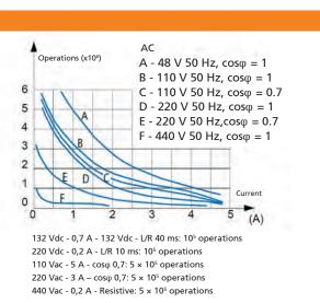
(1) Switching frequency 1,200 operations/hour, 50% cycle.
