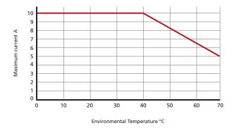
Note: reduction of 30% on all the contacts simultaneously.
