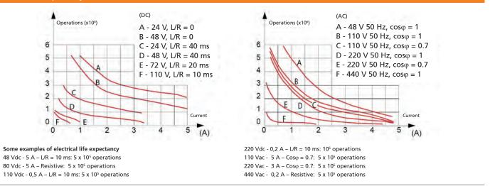
(1) Switching frequency 1,200 operations/hour, 50% cycle.
