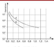
Contact loading: 110 Vdc, L/R 40 ms Curve A : RGM.x7 Curve B : RGM.x3-4-5(NO/NC contact excluded)
