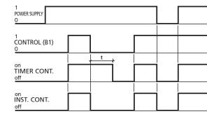
Drop-out delay RDT.x2c-x8c
