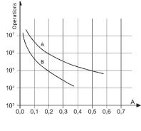
Contact loading: 110 Vdc, L/R 40 ms Curve A : RCM.x6, RDM.x6 Curve B : RCM.x2, RDM.x2
