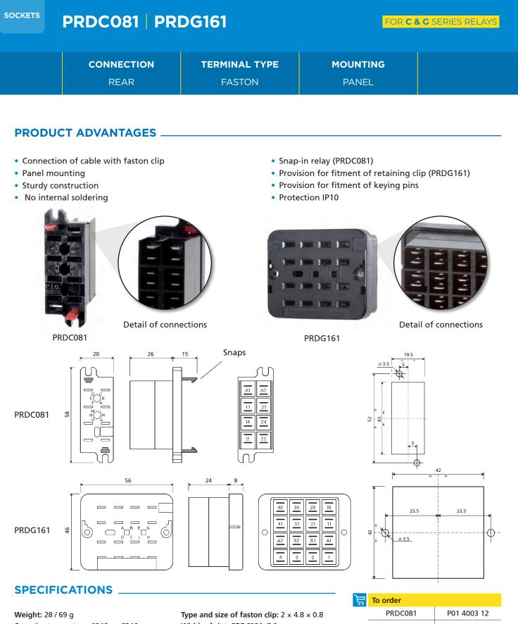
Operating temperature: -25 °C ... +55 °C Storage temperature: -40 °C ... +70 °C Panel mounting: • ø holes: 3.5 mm Degree of protection: IP10 Dielectric strength: 2.5 kV 50 Hz 1 min Width of slot: PRDC081: 7.3 mm PRDG161: 7.8 mm Maximum section of cable: 2 × 2.5 mm<sup>2</sup> Fire resistance: EN 60695-2-1, UL94 - V0 Standards: EN 60255, EN 60947, EN 61810
