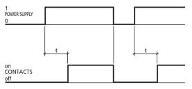
Pick-up delay RDT.x1c-x7c
