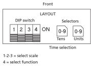
OFF = Pick-up ON = Drop-out Plate is placed on the front of the cover.
