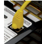
Ethernet output (Modbus TCP) RS485 output (Modbus/Jbus RTU)
