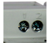
Line termination resistance integrated directly in the RS485 module
