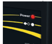
POWER LED: power supply presence (fixed: reset, flashing: battery fault)
