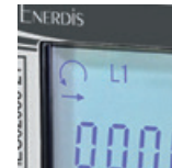
4 quadrants metering with energy balance indicator
