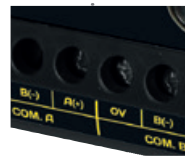
2 x RS485 ports (Modbus/RTU bus) Master mode
